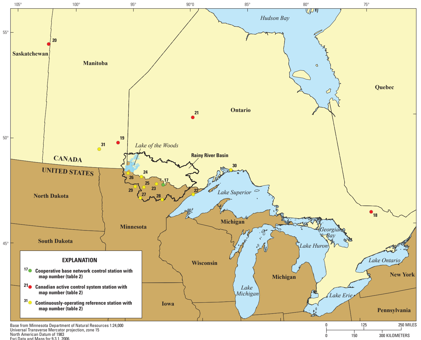
Figure 2. Locations of the National Geodetic Survey cooperative base network control station, Canadian Active Control Stations, and Continuously Operating Reference Stations used to postprocess data collected from global navigation satellite system receivers in this study.
