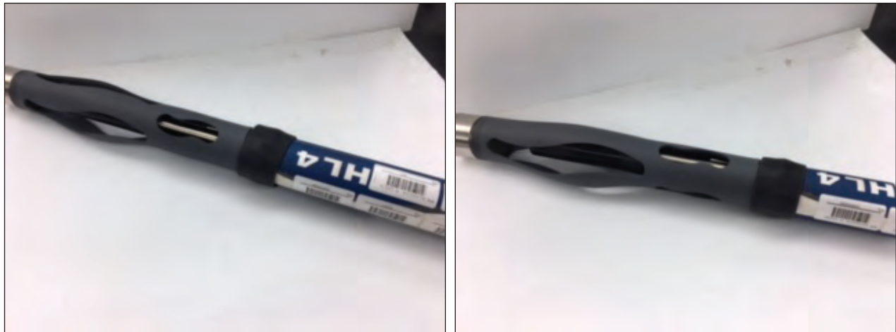
Figure 2. HL4 sonde with warped sensor guard after the initial ramped temperature test.
