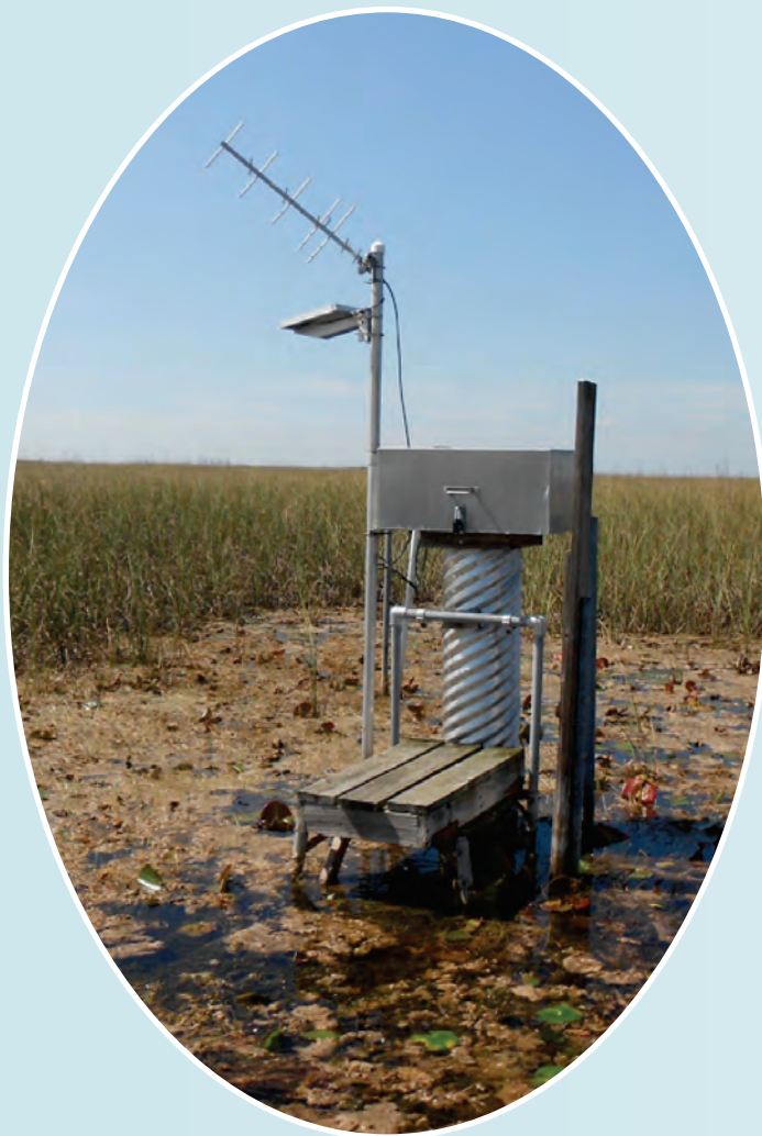
Figure 4. Field water-level monitoring gage EDEN 13. Photograph by Michael Oliver, U.S. Geological Survey.
