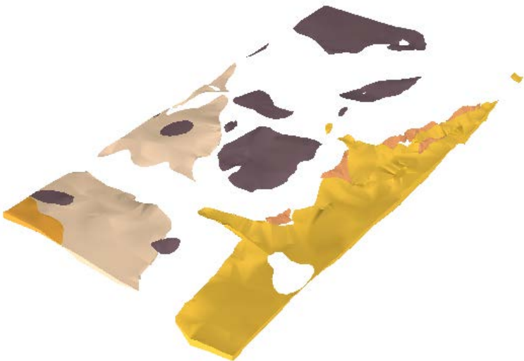
Figure 8 3D view of the river terrace deposits and Langley Silt, looking from the south-west. Alluvium is removed to enable the Shepperton Gravel to be seen (vertical exaggeration x8). Key as per Table 1
